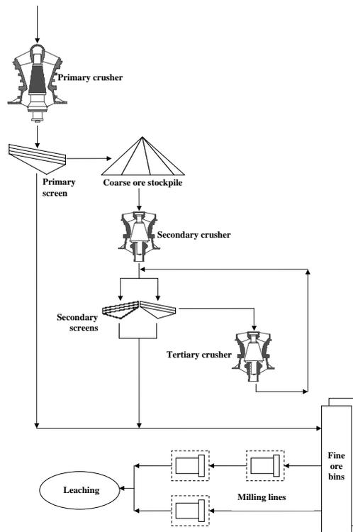
Fig. 1. The basic comminution circuit used in this study.
